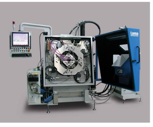
LamaCaster range of multi-slide machines covers all user needs for the production of small precision zinc die castings and can be used for component manufacture for a broad spectrum of industries.
